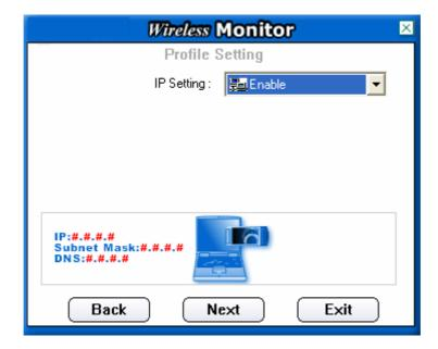
Please define if the current Profile IP setting will be assign by a DHCP Server or just assign by a fixed IP that is determinate by the Network Administrator.
