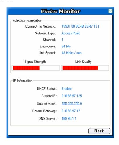
This field is used to display the current status of connection. The state shows "Connected to Network" means normal flow of operation in Infrastructure mode. The PC is connected to access point. Networking is available.
